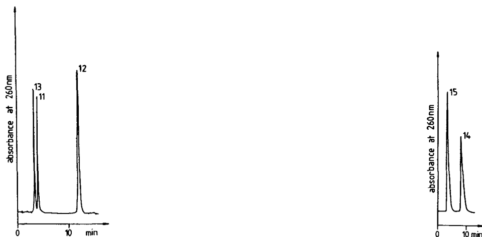
Fig. 10. Chromatogram of 3-trifluoromethyl- \alpha -ethylbenzhydrol and its derivatives obtained on column I. Mobile phase: methanol-0.005 M KH_2PO_4 buffer (70:30, v/v); flow-rate, 1.00 ml/min; column, Hypersil ODS ( 5\ \mu m ) (250 \times 4 mm I.D.); detection, 260 nm. Measured ( m t_R ) and predicted ( p t_R ) retention times: m t_R = 3.70 min, p t_R = 5.0 min for 13; m t_R = 4.37 min for 11; m t_R = 12.74 min, p t_R = 9.9 min for 12.
